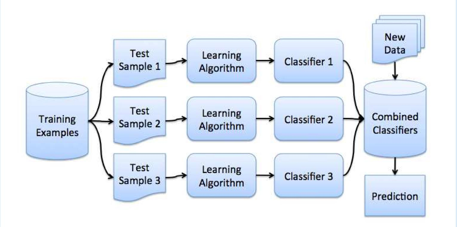
Bagging [4] is a technique that trains various models on different samples of the data and combines the predictions.
