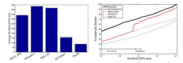
Figure 7: Left: Average runtime; right: runtime CDF for different solvers on ALL; the average feature computation time was 6.7 CPU seconds (shown as a white box on top of SATzilla07's runtime bar). All other solvers' CDFs are below the ones shown here.
