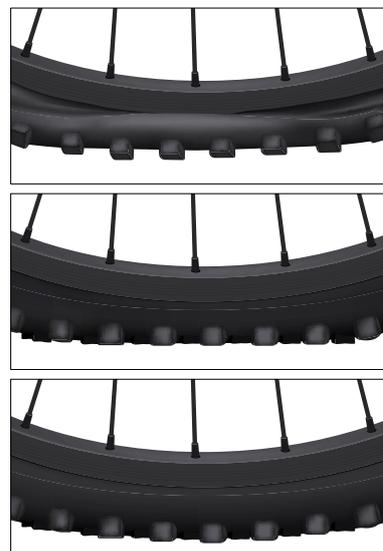
Figure 1.2: Different tire pressures. Top: Under pressurized/flat tire. Middle: Tire with appropriate pressure and good traction. Bottom: Over pressurized tire with low traction.
