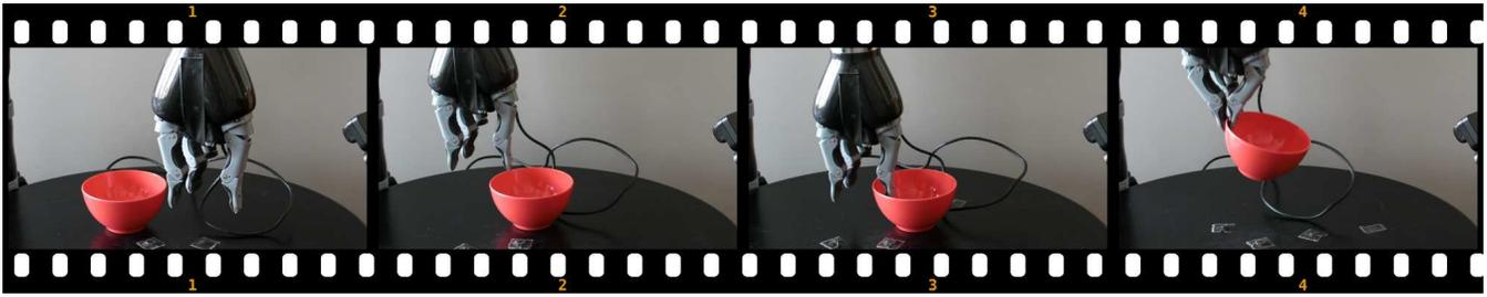
Fig. 7. An example grasp sequence performed by the final system on a moving object.
